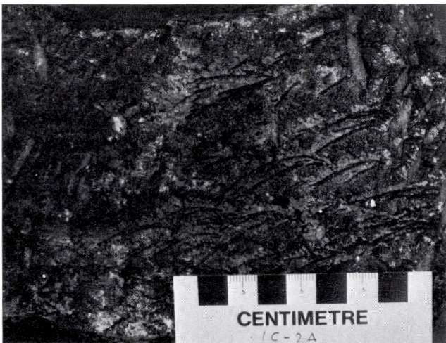
Fig. 13. Dendritic pyroxenes with repeated nucleation along the growth direction.
