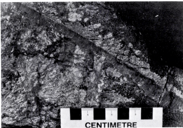
Fig. 23. Dendritic feldspar showing curved growth morphology. Convex, lattice planes can be recognized from the weakly discolored, transverse pattern on the feldspar stem. The crystal measures 18 cm. Secondary nucleation of pyroxene and nepheline on the upper surface tends to readjust growth towards the maximum heat flow.
